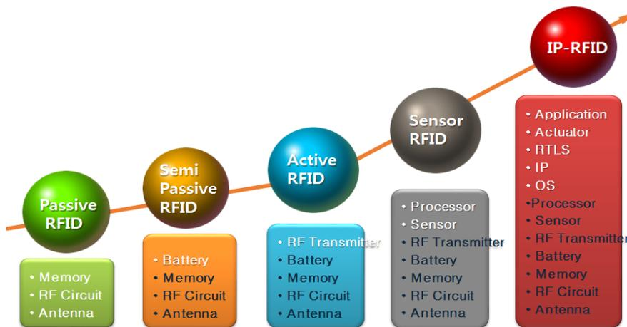
Figure 1. The Functional Differentiations of IP-RFID
