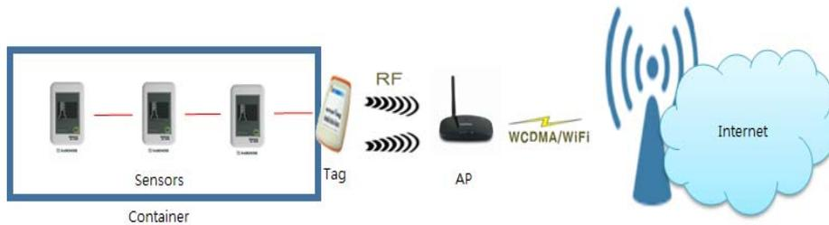
Figure 2. The Separated Type of RFID Tag and Access Point
